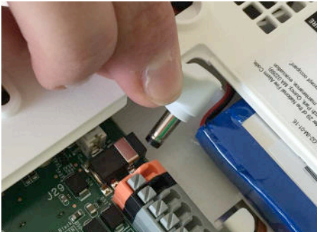
Plug in the power connector
