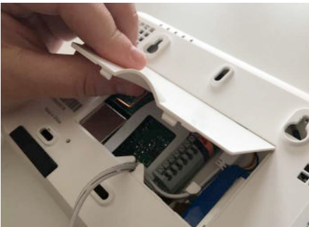
Place the top of the cover onto the panel's back plate
