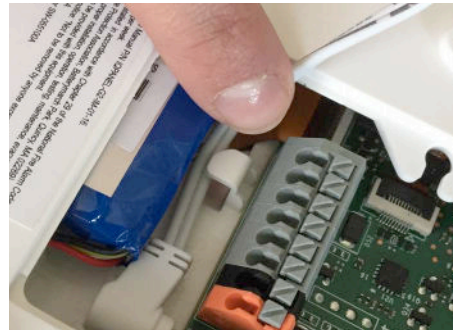
Route the wire behind the retainer clip
